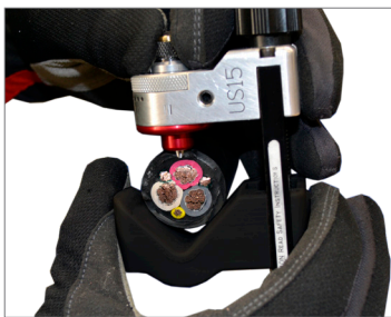
Quick-adjust jaw accepts hard & soft insulated cables ranging from 0.39" to 1.96" (10 mm to 50 mm).
