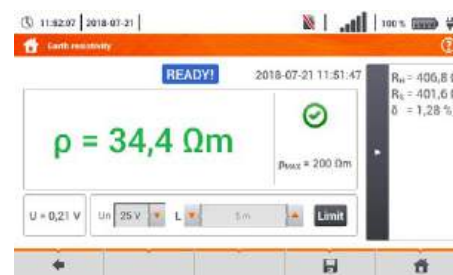
Ground resistivity measurement
