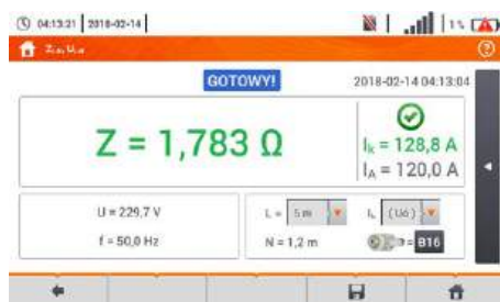
Fault loop impedance measurement
