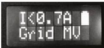
Operation in medium-voltage mode - the display reads the value of the set alarm threshold and indicates the battery charge status
