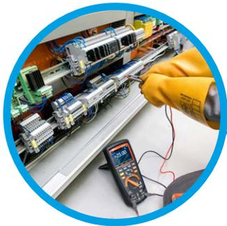
Measurements of the current loop 4-20 mA in analogue circuits controlling temperature, pressure, humidity or flow sensors are possible thanks to the special function that displays the percentage results for the corresponding current values.
