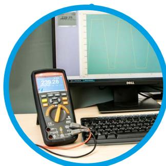
Thanks to the dedicated software **CMM-60 Multimeter Software**, it is possible to transfer results from the meter's memory to a computer program and analyse these results further.
