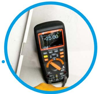
Visibility in all conditions and reading at a wide angle are possible thanks to the colour display with a resolution of 320 x 240 pixels and a diagonal of 3.5".
