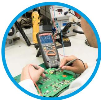
The meter allows the measurement of very small currents in the range of **500 µA**, useful during service works, e.g. in tests of real-time clock support systems or in the maintenance of flame sensors in combustion chambers.
