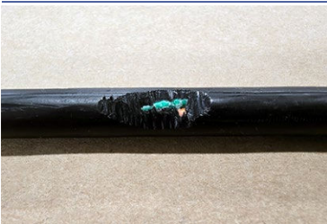
Identify cable jacket defect
