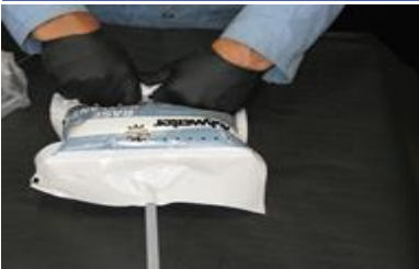
Bursting secondary seal
