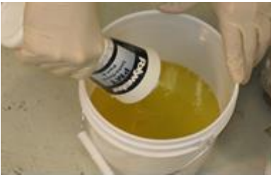
Pour 1 bottle Part A, then 1 bottle Part B into mixing pail
