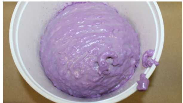
Photo 16: Polywater AFT too hot. Cured quickly.
