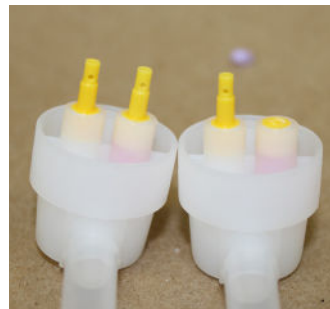
Photo 10: Good nozzle on the left. Broken nozzle on the right.
