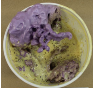
Photo 5: Can held right-side up. Polywater AFT is poorly mixed. Full can dispensed.
