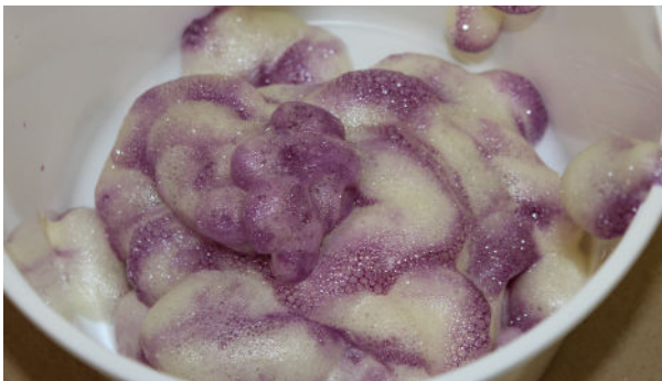
Photo 15: Polywater AFT too cold. Did not mix.
