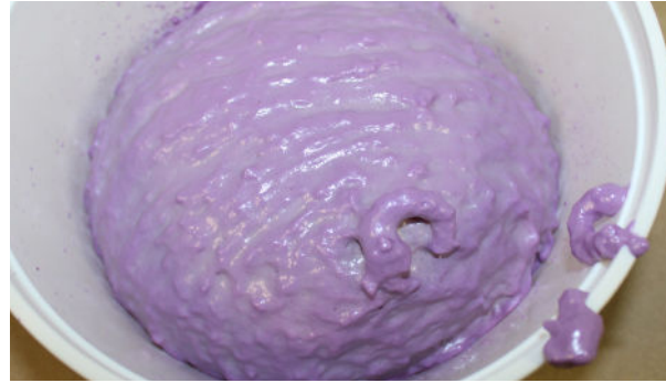
Photo 2: Cured Polywater AFT allowed to rise freely, in bucket
