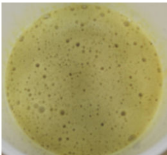
Photo 8: Creamy tan Part A Resin only, Part B side plugged or insert broken.
