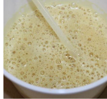
Photo 7: Can held right-side up. Second part of Polywater AFT comes out white Part A only.
