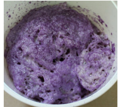
Photo 14: Polywater AFT with no tube on nozzle.
