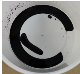
Photo 9: Part B Dark purple Curing Agent only. Part A side plugged or insert broken.
