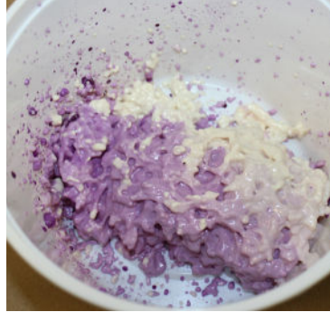
Photo 6: Can held right-side up. First part of Polywater AFT comes out purple but not mixed properly.
