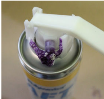
Photo 13: Plugged tube popped off nozzle.
